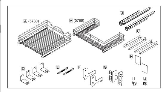
Basket (A), Slide (B), Side mount bracket (C), Bottom Mount bracket (D), Logo cap (E), Mounting bracket (F), Door mounting bracket (G), Double sided tape (H), wood screw (I), Machine screw (J)
