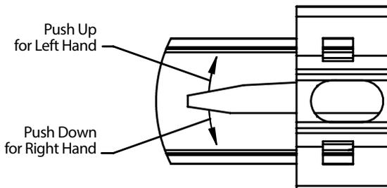
To disconnect drawer member, first extend the slide fully and then lift up the left hand side disconnect lever and push down the right hand side disconnect lever and pull the drawer member out.
